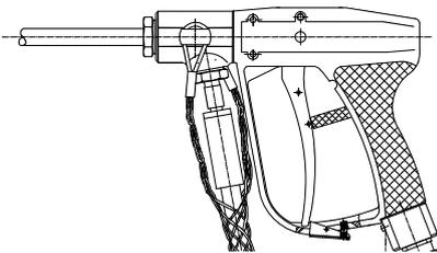
Secure the high pressure hose **every time** with hose protections at the working tool!
