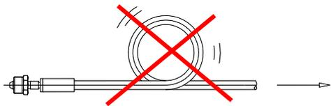
Avoid looping ! After looping during work, shut down the high pressure equipment and carefully remove loop.
