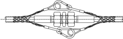
Secure connections of high pressure hoses **every time** with hose protections !
