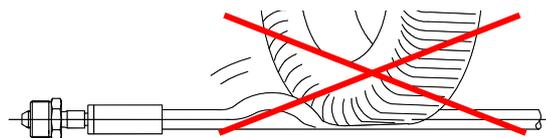
**Never** put weight on the high pressure hose. Use hose bridges, when you have to drive over hoses.
