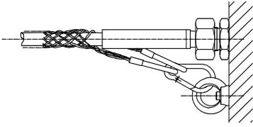
Secure the high pressure hose at the equipment **every time** with hose protections!
