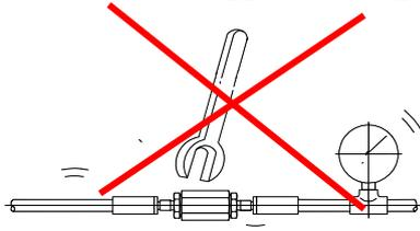
**Never** tighten fittings of high pressure hoses under pressure !
