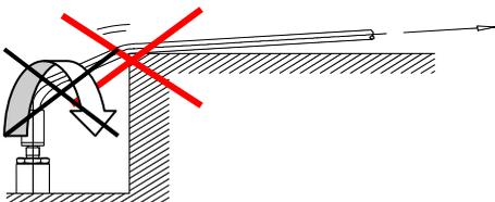
Do not bend high pressure hoses or pull them around sharp edges. At work on edges or several floors coat hose or edge. Do not bend fitting.
