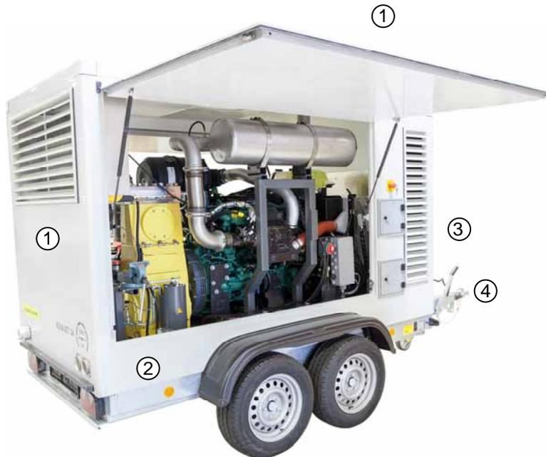
Road going 14 series units for use on public roads are mounted on a tandem axle trailer with overrun brakes. They conform to the German TÜV regulations. Height adjustable ring or ball type couplings are available on request.
