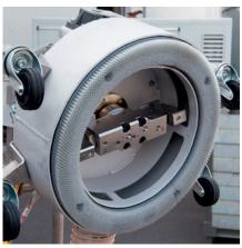
Oscillating movement for optimal treatment of localized damage. Totally covered jetting area for high safety and possibility of environmental friendly vacuuming of waste water.
