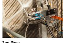
**2nd Gear**Medium pump power for pipe and tube bundle cleaning
