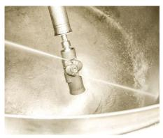
**3rd Gear**Full pump power as typically employed for tank cleaning
