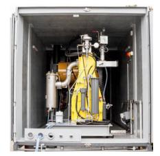
"S Class" and "Aquajet" units can be built into 20 ft. or 25 ft. sound damped containers, sound damped aluminium truck bodies or trailer containers (BDF).
