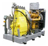
"S Class" and "Aquajet" units can be built into 20 ft. sound damped containers, sound damped aluminium truck bodies or trailer containers (BDF).
