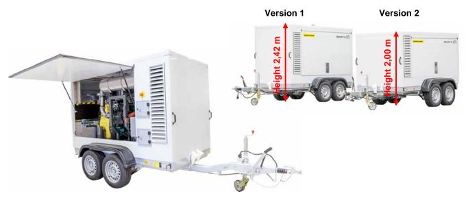
The high pressure pump units are built to be reliable and user friendly.
