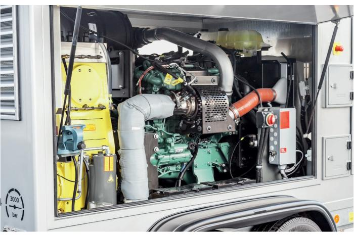
Mobile unit driven by diesel engine with AdBlue® system
